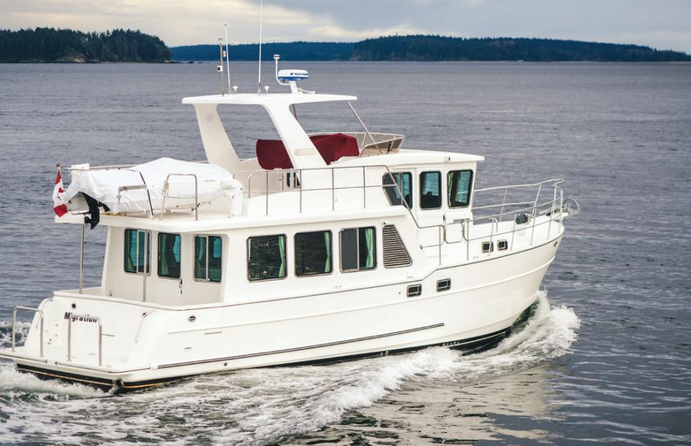
Our noise meter registered 64 decibels. We throttled up to 2000 revs for a two-way run to negate the current conditions in British Columbia's Fraser River, where part of our test was done. Average speed was 8.4 knots, and our noise was 73 decibels. At wide-open throttle, 2680 rpm, we made 11.1 knots while burning 10.9 gph.
